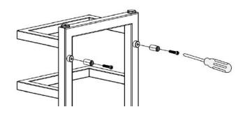
5. Align and push the rail brackets on the radiator onto the wall brackets secured to the wall. Secure the two together with the connecting screws provided (insert through the slot in the bracket) and tighten by the Philips screwdriver, be sure not to overtighten.
